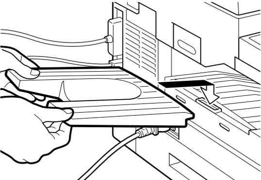
A line drawing showing a hand placing a delivery tray onto a device. The tray is being aligned with a slot on the front of the device. The tray has a handle and a series of parallel lines on its surface. |
