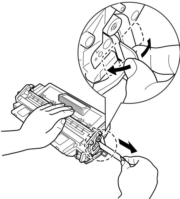
A line drawing showing a hand holding the cartridge. A circular inset provides a magnified view of the internal mechanism. In the inset, a hand is shown pulling a small tab away from a component, with an arrow indicating the direction of movement. Below the inset, a hand is shown pulling a thin tape out of the cartridge, with an arrow indicating the direction of the pull. |
