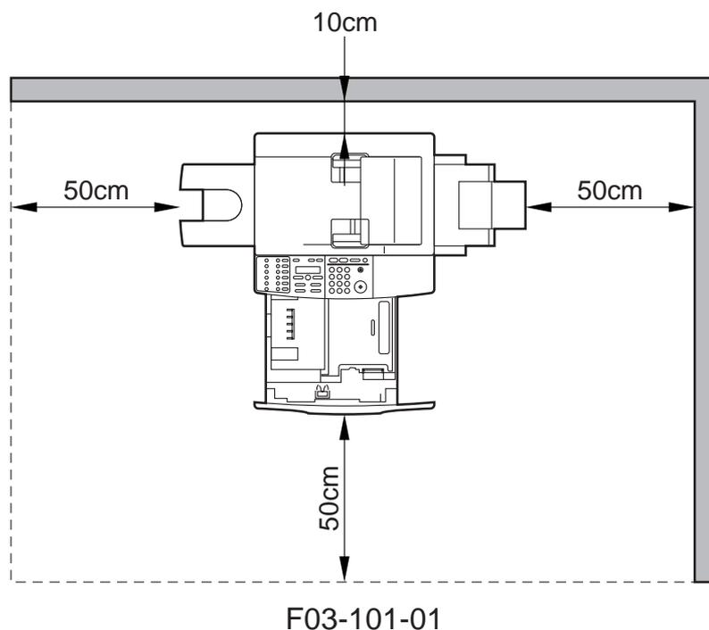
6. The machine will have to be placed in a well-ventilated area of the room. Do not, however, place it near the inlet of air.
