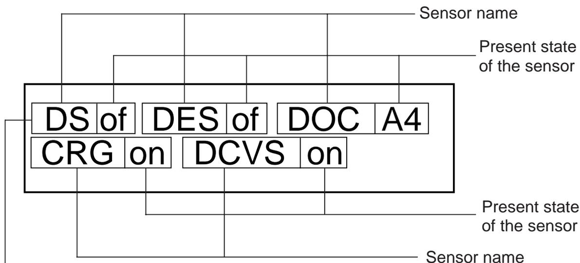
'DS of' indicates that the original sensor (DS) of the ADF is OFF.
