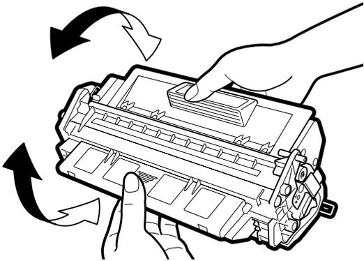
A line drawing of a hand holding a rectangular cartridge. Two curved arrows indicate the rocking motion from left to right and right to left.                                                                                                                                                                                                                                           |
